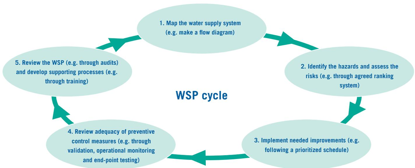
Figure 1 – Water Safety Plan (WSP) cycle
